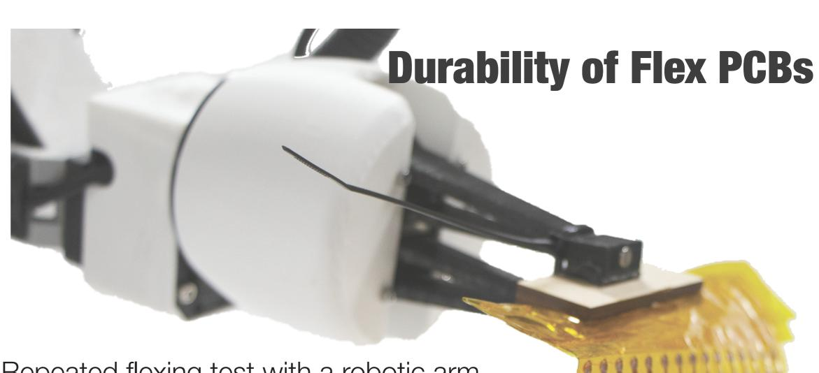
Repeated flexing test with a robotic arm. 20 circuit traces of 0.5mm, 1mm, and 2mm (kapton: 90 microns, copper: 38 microns)
