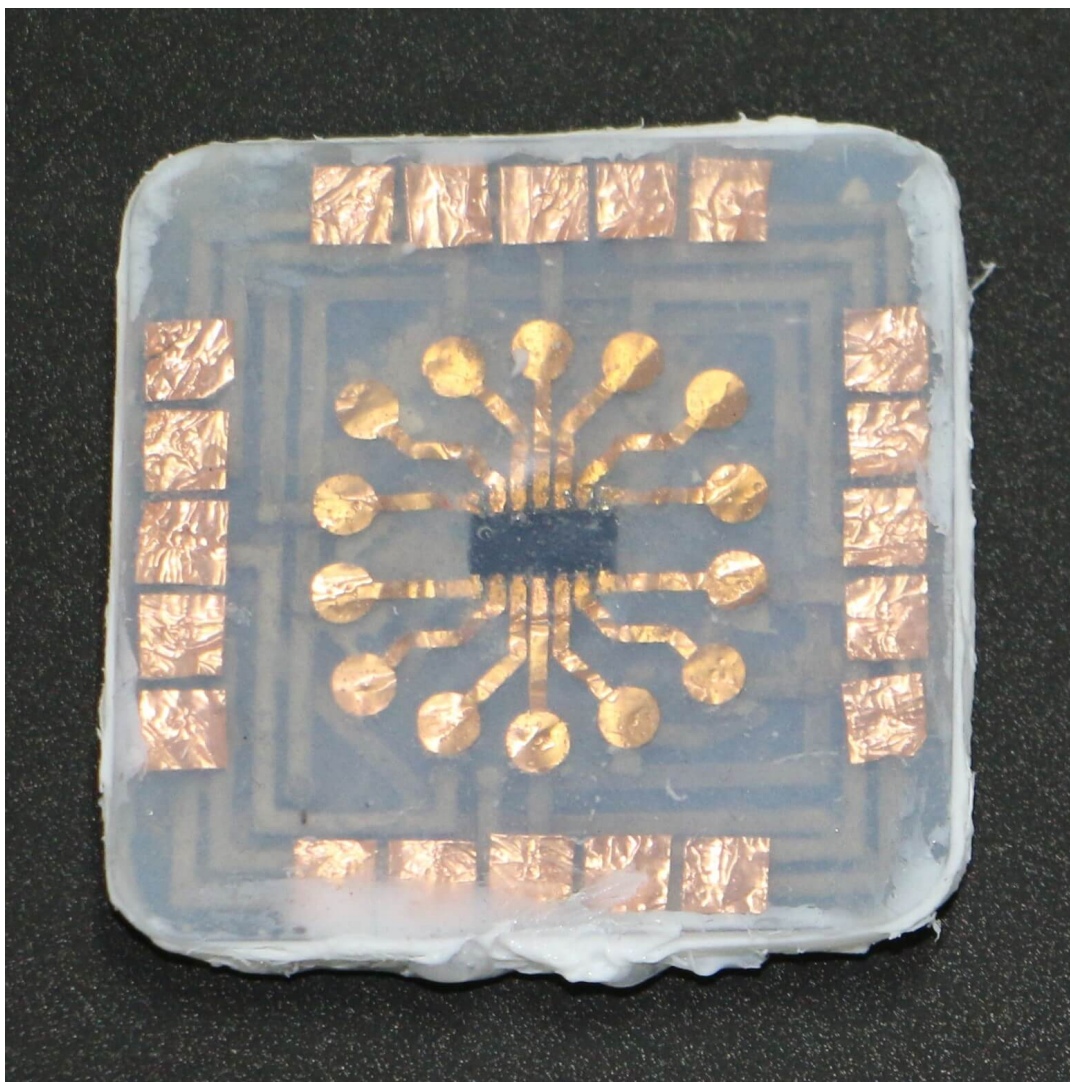
FIGURE 4.9: First iteration of the fabrication of modules using a copper extension pad and Galinstan.
