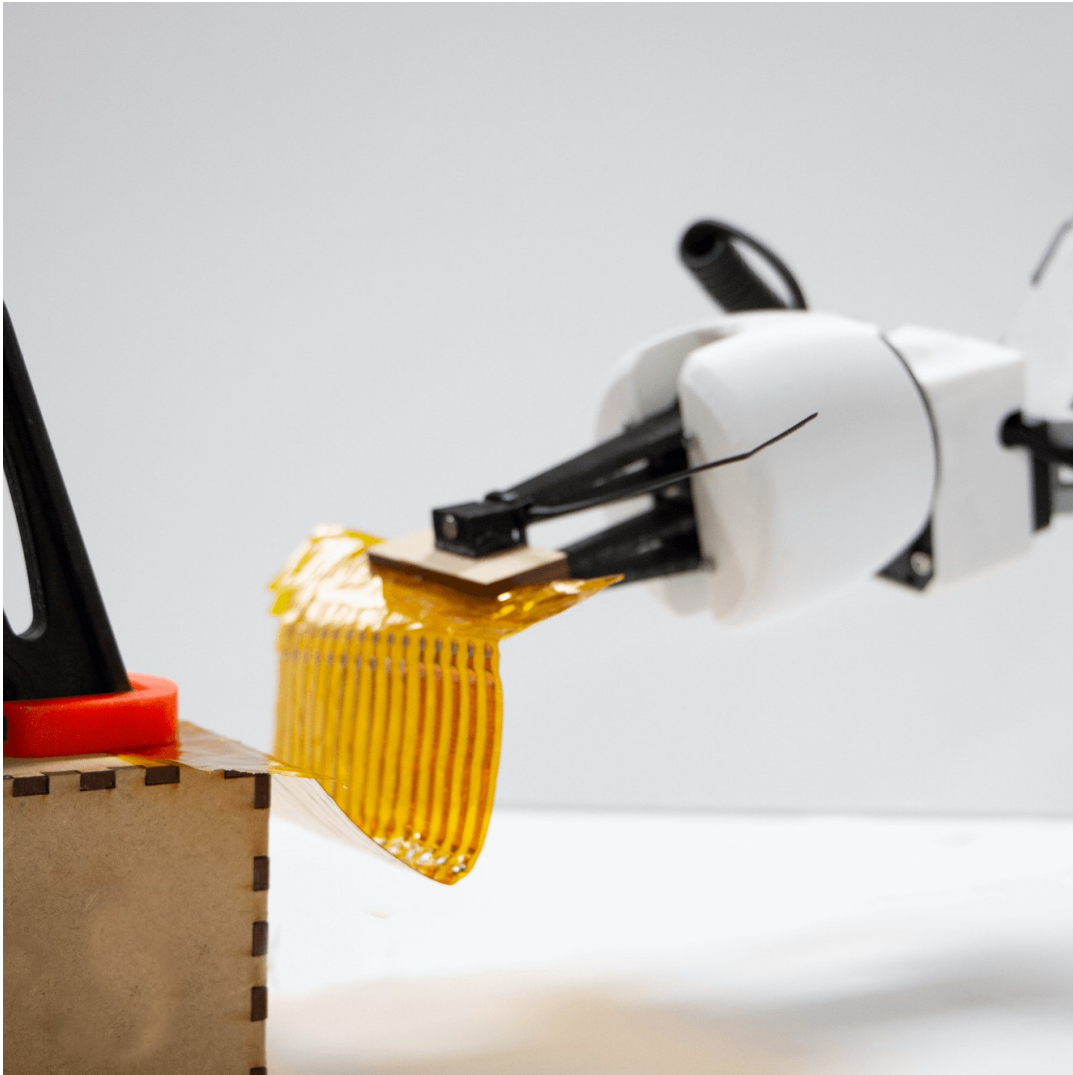
FIGURE 5.8: Stress test of the PCB using a robot arm.
